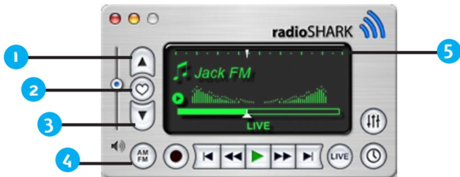
1. **TUNE UP** - Pressing the Tune Up button increases the frequency by one step according to the settings selected in the Tuning section of the Preferences. The frequency will continue to increase until the Tune Up button is released.
